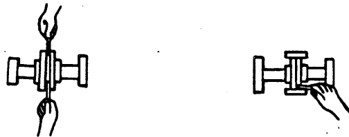
Figure 3B. Aligning Non-Spider Type Couplings
