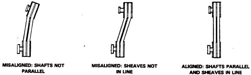
Figure 3C. Alignment of V-Belt Driven Pumps
