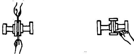
Figure 3B. Aligning Non-Spider Type Couplings
