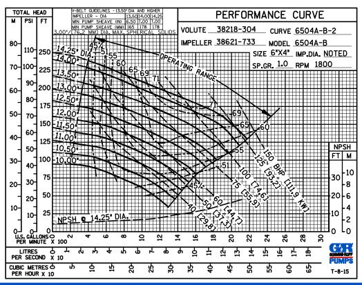
50 HERTZ PERFORMANCE BASED ON WATER TRIMMED IMPELLER
